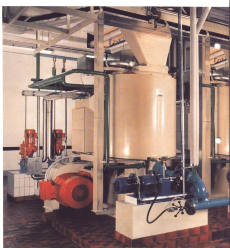
vessel is flanged directly onto the lower stirrer drive gearbox which doubles as the machine base.
